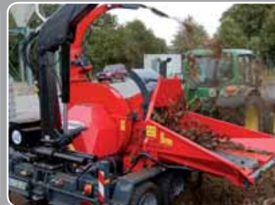
JT600 equipped with a conveyor belt of 2300 mm and a crane.
