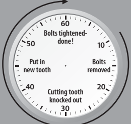
Changing the cutting tooth in 60 sec.
