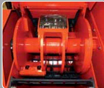
Rotor diameter 600 mm with 6 chipping blades and large flywheel.
